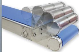
**Flip-Up Tail** releases tension on the belt for easy cleaning. Flip-down stand brackets in tandem with the flip-up tail allows for quick belt removal for in-depth cleaning.
